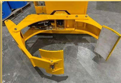
LRCR Outer Position Clamping range 24" (61 cm) to 40" (102 cm) in diameter.
