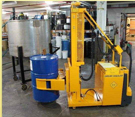
RCR1324-8 with Adapter Reduces the clamping range to 8" (20 cm) to 19" (48 cm) in diameter
