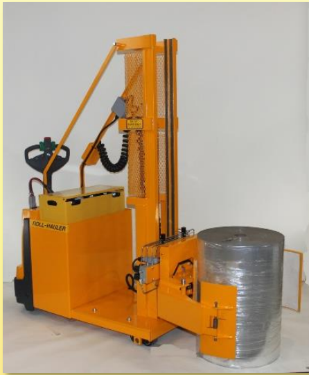
RCR1626-16 with FDA metallic grey powder coating in open position
