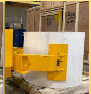
LRCR Clamp picking or placing a vertical roll
