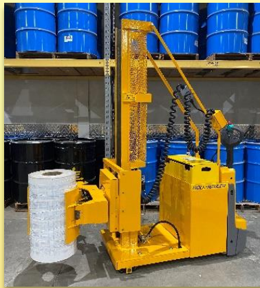
SRCR Outer Pin Position Clamping range 18" (46 cm) to 26" (66 cm) in diameter.
