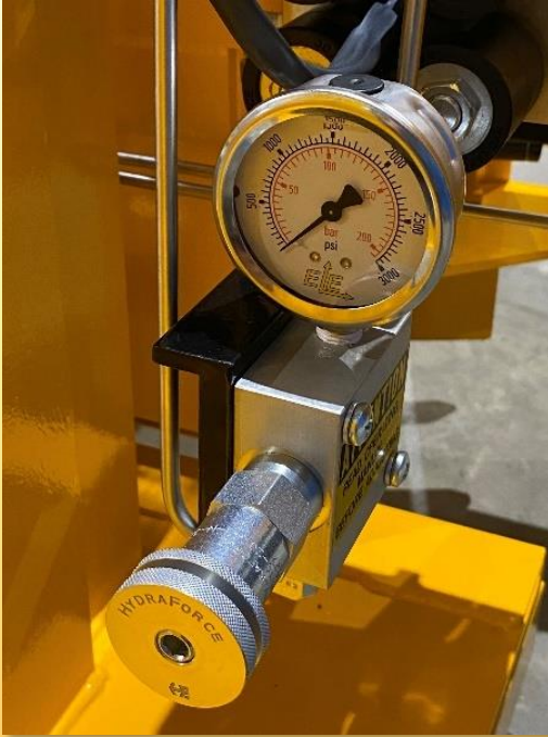
Side-Rotation Adjustable Clamping Pressure
