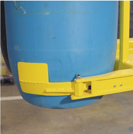
Mechanical clamping arms hold drums securely while unloading
