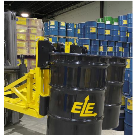
Double gripping heads are best for light gauge open head drums
