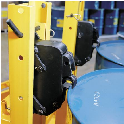
Heads adjust vertically for handling shorter height drums
