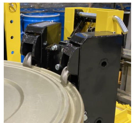
Double gripping heads are best for light gauge open head drums
