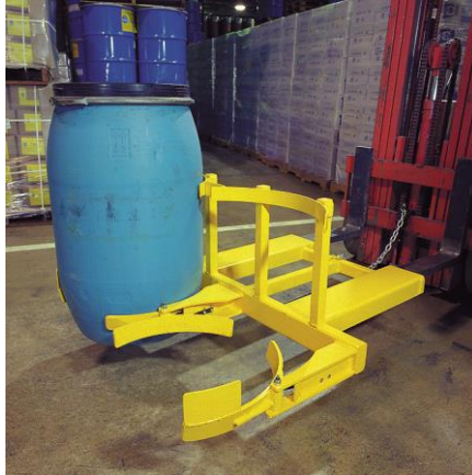
Can grip one drum on either side or both drums together
