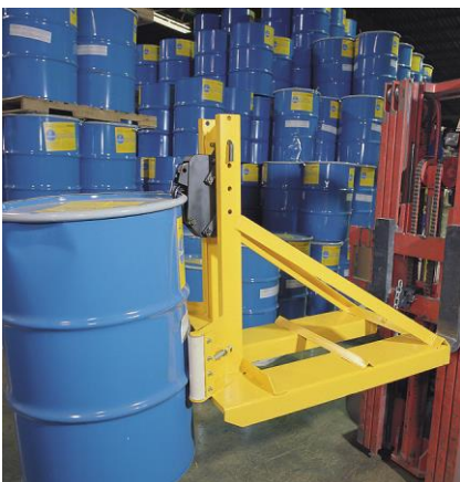
The model EG3SCM-NF has a narrow 24" overall width to grip drums in tight areas or pallet racks
